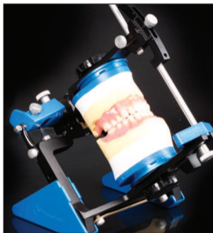
Figure 6: Completed upper and lower dentures on the Panadent PCH articulator
